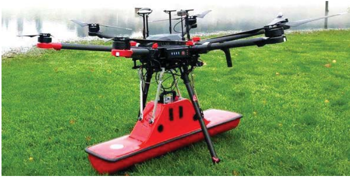
Figure 4 - Drone-based Ground Penetrating Radar (GPR)
