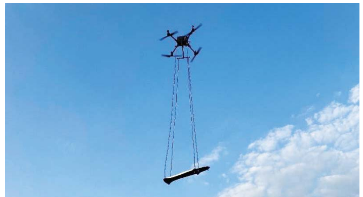
Figure 1 - Drone-based Magnetometer – MagArrow
