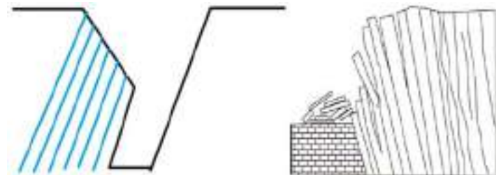
Fig.6 Major joint set present in the hangwall and possible failure mode
