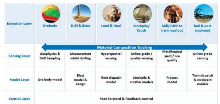
Fig 4: Various Industry 4.0 layers covering mining process
