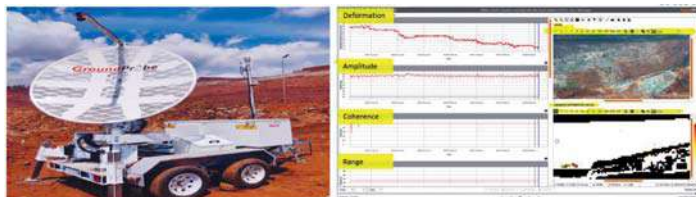
Fig 17: Real Time Monitoring through Slope Stability Radar
