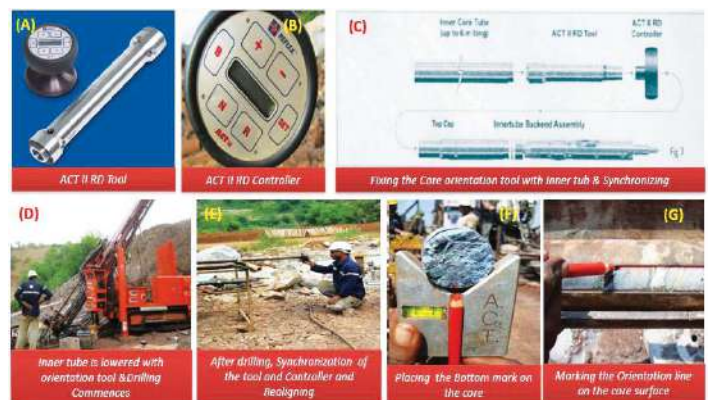
Fig 8: Digital core orientation technique
