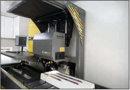
Hyperspectral Core Imager (HCI) integrates high resolution VNIR-SWIR imaging spectroscopy, core photography and 3D laser profiling to deliver the most advanced automated core logging system.
