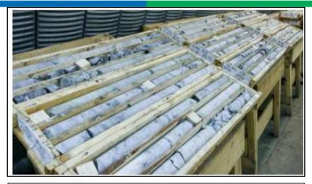
XRF analysis allows for the determination of rock cores elemental composition. The ability to carry out XRFbased rock core analysis at sites of interest enables mineral exploration assays to be performed without having to transport heavy samples to a different analysis site. As the analysis can be done automatically a quick and thorough assay of all samples is possible with reduced personnel workload and analysis time.
