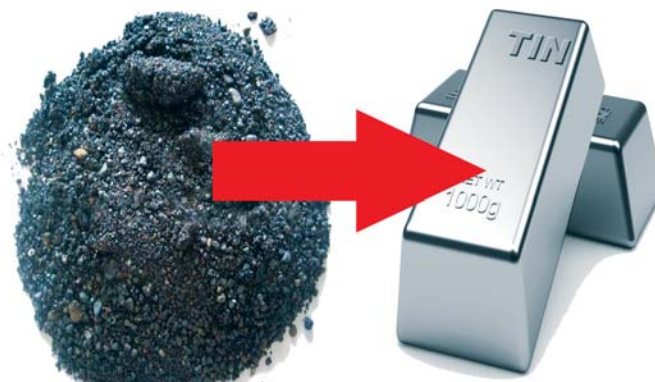
Fig. 4. Cassiterite, the tin oxide, dark black, earthy non-good looking ore mineral concentrate when smelted produce eye catching attractive silvery white metal.
