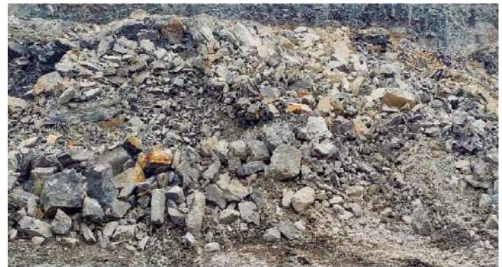
Blast performance without stemming plug
