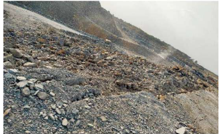
Blast performance with stemming plug
