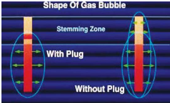
Figure-4. Possible Mechanism causing blocky collar
