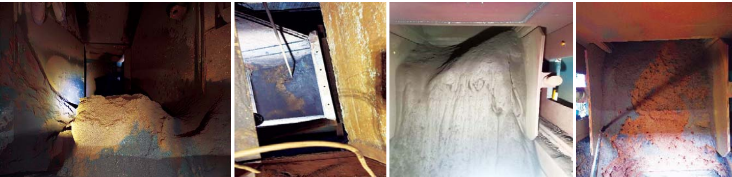
Fig. 1.2 – Intermediate chutes jammed by the clumping of limonitic, lateritic and blue dust types of iron ore
