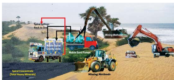
Fig. 7. Suggested proposal for different mobile mining methods and mobile spiral concentrators for recovery of total heavy minerals along the coast.
