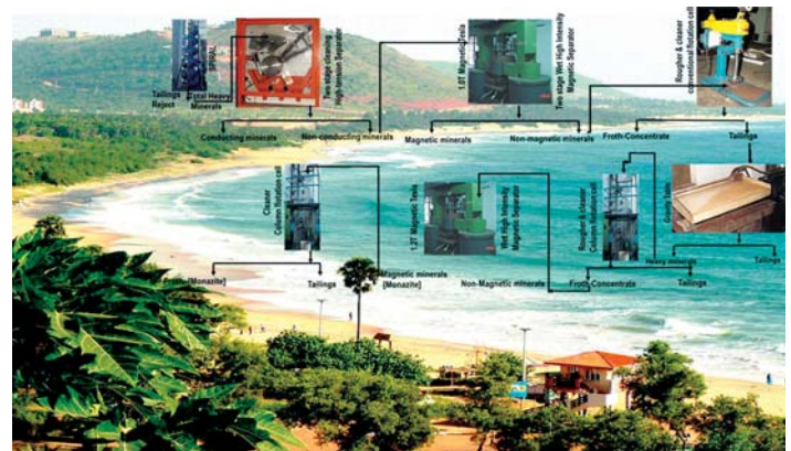
Fig. 2. Experimental procedure to recover placer rare earth mineral from beach sand monazite
